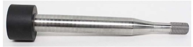
Tensile Nut Proof Load Test Fixture
