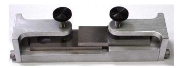
Model No. ASTM.F1044.30 Specimen Size or Difference Between Fixtures 1" wide by 3" long lap shear panels
