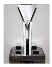
Model No. ASTM.D5041.10 <u>Specimen Size or Difference Between Fixtures</u> 6" wide, up to 0.25" thick and 6" long
