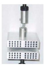
Model No. ASTM.D3354.10 Specimen Size or Difference Between Fixtures 4" wide by 7" long, any thickness <u>Construction</u> Aluminum with protective finish Temperature -20 to 120°F (-29 to 49°C)
