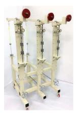
Model No. ASTM.D2990.103AT Specimen Size or Difference Between Fixtures Construction Up to 1" wide and 0.25" thick
