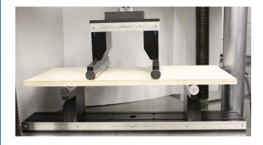
Model No. C0158.40 Specimen Size or Difference Between Fixtures 34" by 5" wide
